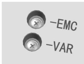
Schematic Diagram of Stop Screws of Ironclad Cabinet
